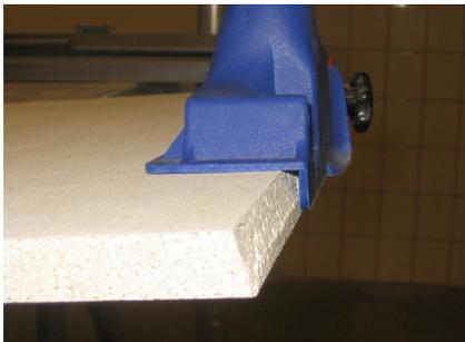
Detail edge plane on the visible side
